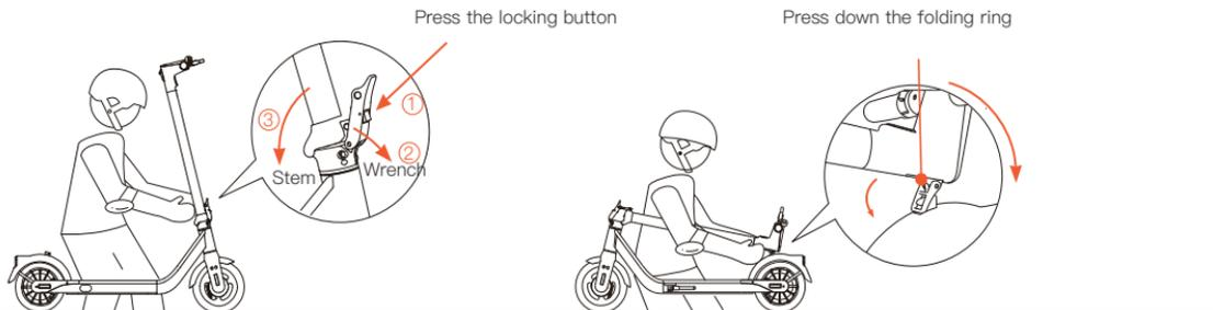
Power off the scooter, hold the stem, press the locking button and pull the lever, bend the handlebar stem towards the footrest.
