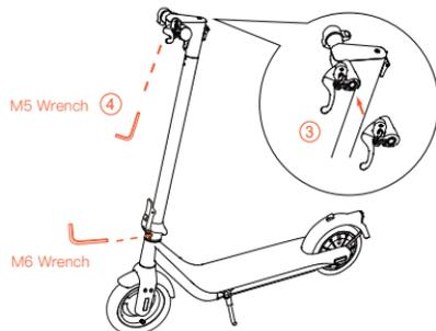
3. Place the brake lever on the handlebar, tighten it firmly with hex wrench to be sure it won't loosen.
