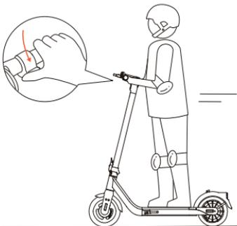
3. Stand on the footrest with both feet, press the throttle on the right hand.
