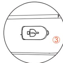
3. Remove the battery charger and close the rubber cap when charging finished.
