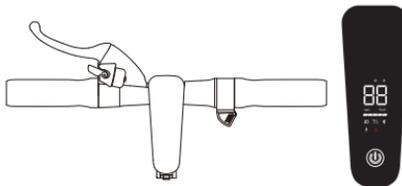
1. Check the power level indicator after powering on. Charge the scooter if the battery level is low.
