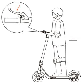
4. Slow down by releasing the throttle and hold the braking lever lightly (Do not brake suddenly and watch out for the road conditions!).
