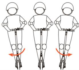
**!** Do not rotate the handle violently while driving at high speed.
