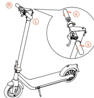
4. Install the handles on the stem and firmly tighten it according to the correct position and direction marked on the label.
