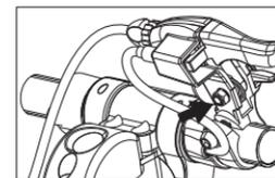
3. Fix the brake lever with M6 hex wrench.
