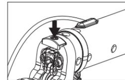
5. According to the shaking condition of the pole, properly adjust the folder screw
