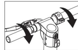
4. Tighten handlebars (Pay attention to the direction of rotation when tighten).
