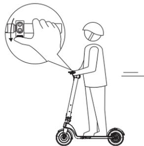
4 Press the THROTTLE button slightly on your right hand to start and rotate the handle to turn
