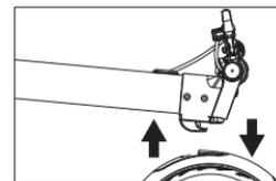
1. Pull up the lever while pressing down the rear wheel fender.
