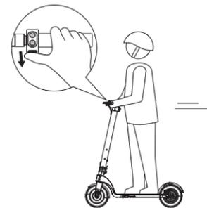
5 Press the THROTTLE button to speed up. Do not ride too fast.
