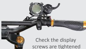
Check the display screws are tightened
