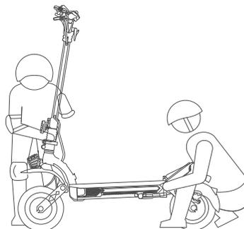
Lift up the bottom of the front fork and rear foot pedal to carry if necessary. Make sure the scooter is carried by two or more people. **⚠ Risk of pinching!**
