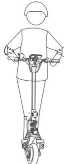
5. To turn, shift your body and turn the handlebar slightly. \* Please watch out for road conditions, sufficient turning space is required.
