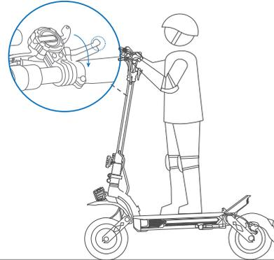
3. Put both feet on the footboard and stand stably. Pull the throttle to speed up. \* This scooter starts at an initial speed of 0 km/h. Note: Disable the Zero start-up feature via the Dualtron app. When disabled, the motor will not engage until the scooter reaches 1.9 mph (3 km/h).
