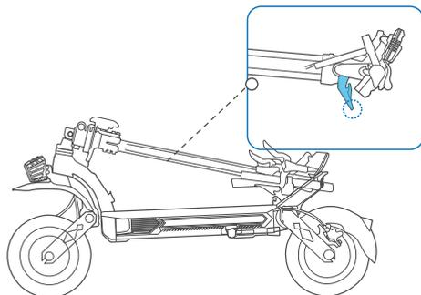
Fold the steering post, lock the steering tube to the deck.
