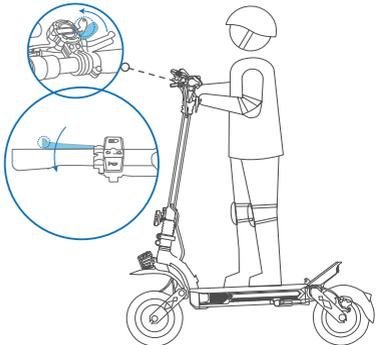
4. Slow down by releasing the throttle and squeezing brake levers.
