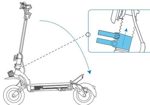
Release the wide QR lever, raise the locking slide upwards.
