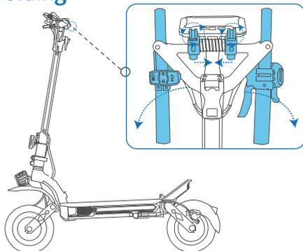
Release the QR lever of handlebar, move the locking slide inward and fold the handles.
