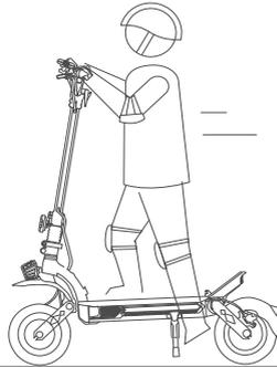
2. Stand on the footboard with one foot and push off with the other foot to start gliding. \* Make sure you have disabled SAFE mode. (SAFE mode setting via Dualtron app. Deactivate safe mode by squeezing brake lever.)
