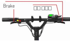
**Caution** Before driving, be sure to check the folding part, the handle part, the part where the main fixing part of the product is fastened well. And check the position of the fixing slide, the QR lever locking status and the folding part fixing status.
