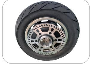
1. After removing the arm endcap, using a 5mm spanner to take out the screws. Then disconnect the motor cable, and disassemble the wheel and motor fastening bolts.
