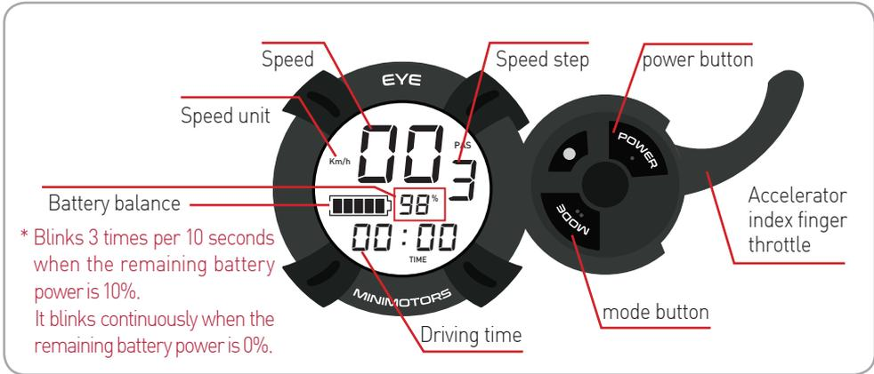
\* Blinks 3 times per 10 seconds when the remaining battery power is 10%.
