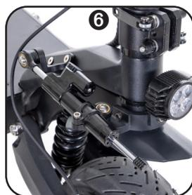
Finally, set the handlebars all the way to the left and then tighten the adjusting screw **9** firmly. The strength can now be adjusted on the adjusting wheel above the steering damper.
