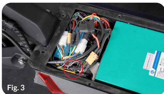
In the cable shaft there are 2 black connectors with black/white cables (Fig.3, 4).
